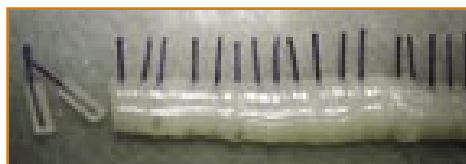
Figure 1. The thread is slid into a 1cm-thick line of adhesive.
