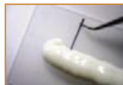
Figure 1. The thread is slid into a 1cm-thick line of adhesive.
