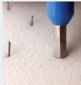
FIGURE 2. Tip “engaged,” ready for punch advancement
